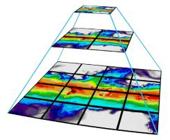
The Grid Elastic Database builds a pyramid of tiles from the gridded data, providing fast access to different levels of resolution. This pyramid structure enables efficient data retrieval for different zoom levels, ensuring users can access gridded weather data at various scales.
